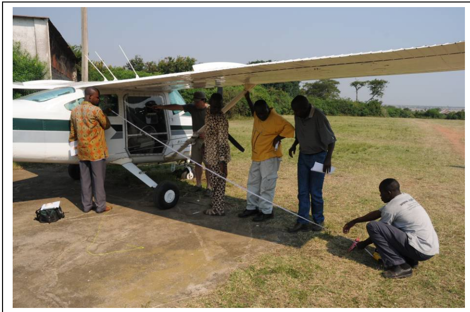
Figure 2. Trainees calibrating the airplane for SRF surveys
